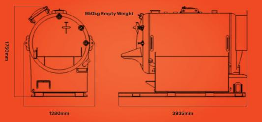
Can be registered with Worksafe as plant equipment **AS1210 CL3 and** AS4343 compliant
