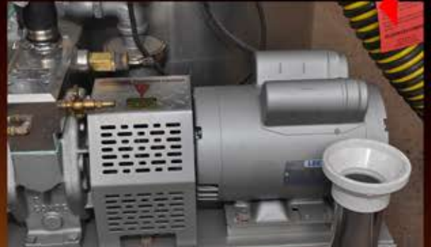
1.5HP ELECTRIC MOTOR
